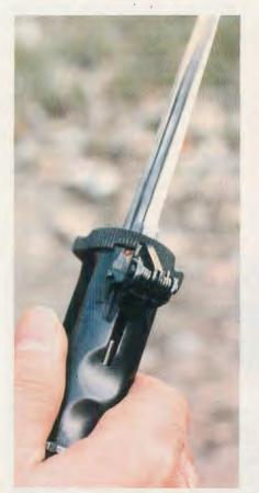
ABOVE: Red dot on safety ring of trigger/crossguard means knife pistol is ready to "fire." Note front sight just to left of trigger pivot and return spring.
